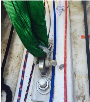
Fig1. Shows secure lifting point within the boat.
