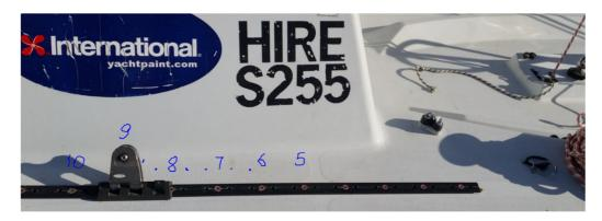
The Genoa car roughly moves a similar amount to the halyard tension, so if you tension the Halyard 100mm as the wind increases, then the Genoa Car will need to move aft 100mm or 2 holes.
