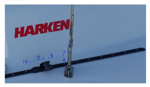
The Jib Car position is shown roughly in a Mid-Range position, screws numbered from the front of the track.
