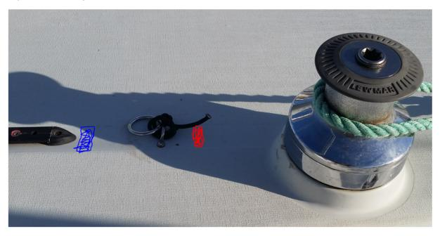
Now sheet the Genoa on until the Mid leech is in line with the Spreader tip (the Foot will wrap firm around the Cap Shroud), and place a tape mark on the Deck under the mark on the Jib sheet for Maximum Trimmed On Position (near Deflector ring or maybe to Red Mark in Photo above). Make sure the leech ribbon, if fitted to upper leech, is flowing.
