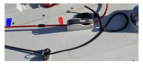
Put a tape mark on the deck as show in Blue in photo. Tape Mark Halyard at the Blue position. This will allow range if you have to increase halyard tension if the wind speed is high, so you can remove stretch. Red mark in front of the Clutch is a possible maximum in fresh breeze.
